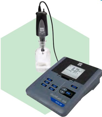
As the direct replacement for the YSI 5000, the MultiLab 4010-1W is most often used in water resource recovery facilities (WRRF) for the determination of biochemical oxygen demand (BOD). A typical 4010-1W configuration includes:
